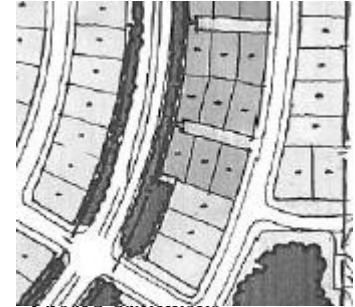
Shared driveways (upper right) abutting arterial
